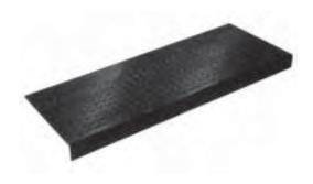
Lo-Disc Stair Tread has 3/4" diameter discs, raised .025"; is an economical, attractive long wearing resilient rubber tread; added gauge at front edge. Tapered discs are easier to clean. An excellent tread for lighter traffic stairways. Meets Federal Spec. RR-T-650E and ZZ-T-001237 (GSA-FSS). Install with Neoprene Contact Flooring Adhesive.
